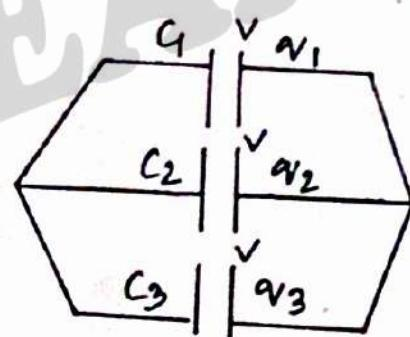
$$\begin{aligned} qV &= qV_1 + qV_2 + qV_3 \\ \Rightarrow CV &= qV + C_2 V + C_3 V \\ \Rightarrow C &= q + C_2 + C_3 \end{aligned}$$
