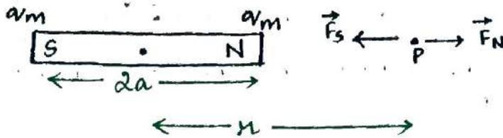
$P$  is any point on the axial line at a distance  $r$  from the centre.
