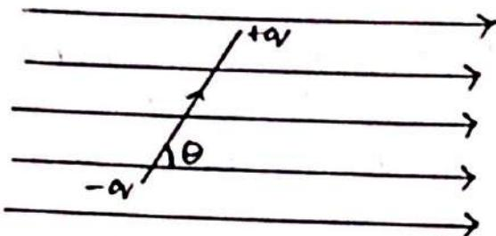
$\theta$  is the angle between dipole moment and electric field intensity.
