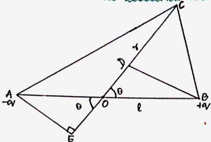
C is any point at a dist  $r$  from the centre of the dipole making an angle  $\theta$ .
