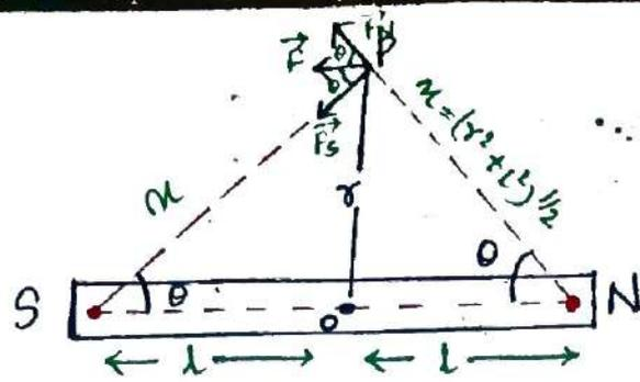
P is any point on the equatorial line at a distance r from the centre.
