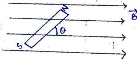
When magnetic dipole is left in uniform magnetic field at any angle, it executes S.H.M
