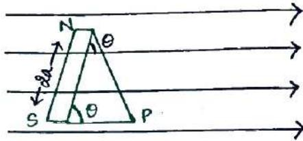
Let the magnetic dipole moved through a small angle  $d\theta$  and torque acting on dipole is  $\tau$ . Then the small work done in moving dipole  $dw = \tau d\theta$
