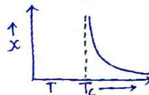
$T_c$  (Curie's temp) - temp above which ferromagnetic substance behaves like paramagnetic substance.
