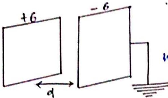
It consists of 2 parallel metal plates separated by some distance having some insulating medium between them. 1 plate is given +ve charge and other plate is connected to earth.
